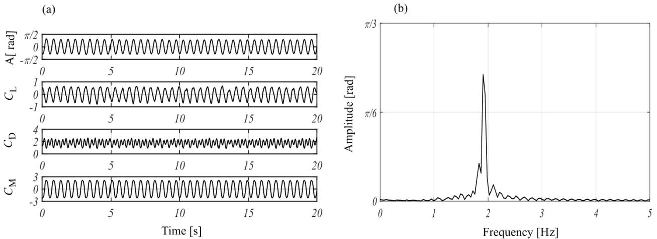
Fig. 1 The time history of amplitude and force coefficient (a). Single-sided amplitude spectrum (b).
