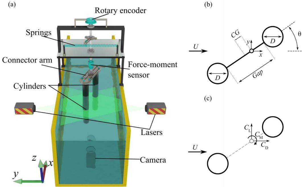
Fig. 2 3D view of the experimental setup (a). A simple schematic diagram of two cylinders (b). A simple schematic diagram of force coefficient where vector shows the direction of force acting on the cylinders (c). Note that the drawing is not to scale.
