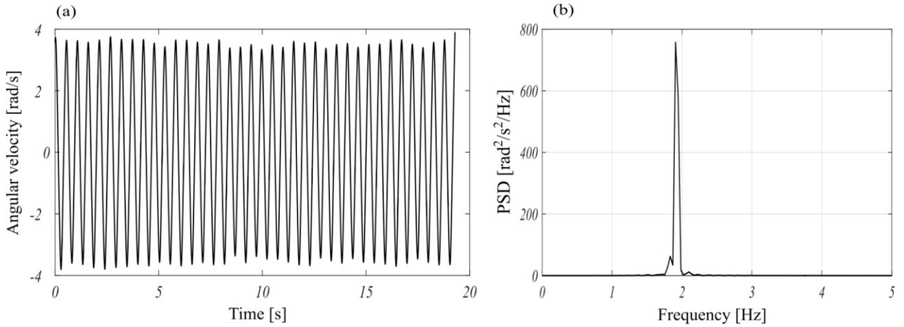
Fig. 3 Angular velocity when  $CG=0$ ,  $Gap=0.9$  (a). The power spectral density of the angular velocity, when  $CG=0$ ,  $Gap=0.9$  (b).
