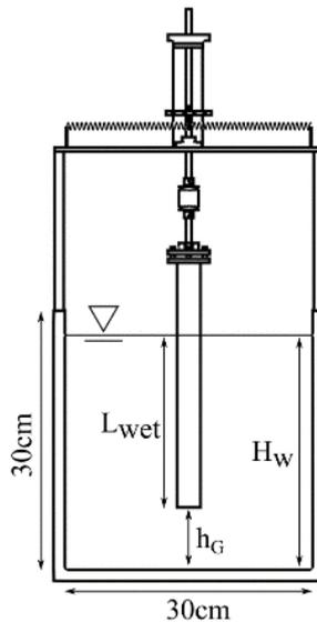
Fig. 2 Front view of the experimental setup.
