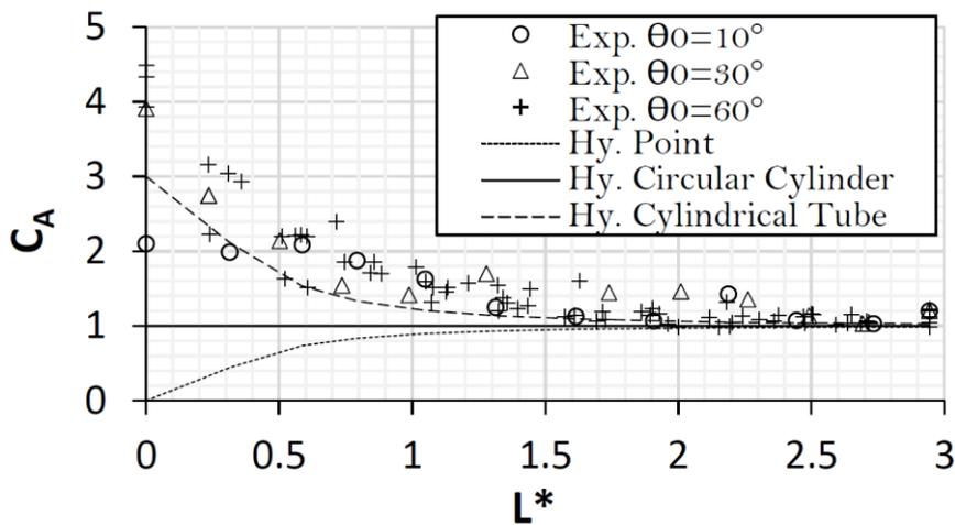
Fig. 3 AMI coefficient ( $CA$ ) as a function of the arm length ratio
