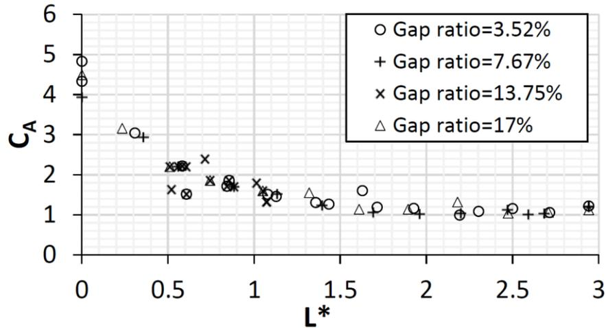
Fig. 4 AMI coefficient ( $C_A$ ) as a function of arm length ratio ( $L^*$ ).  $L_{wet}=0.139$  m and initial displacement is  $60^\circ$ .
