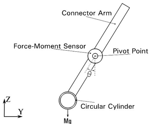
Fig. 3 Side view schematic of the pendulum setup of the apparatus.
