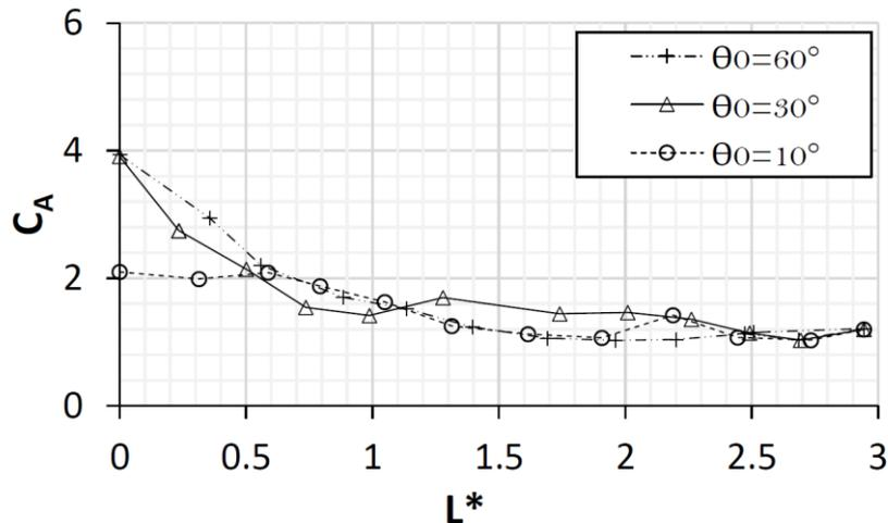
Fig. 5 Experimental results of AMI coefficient ( $C_A$ ) as a function of arm length ratio ( $L^*$ ) for different initial displacements. (gap ratio=18.2%)
