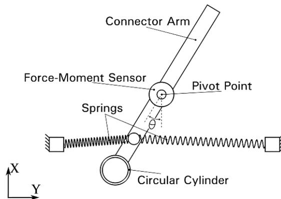
Fig. 4 Plan view schematic of the cylinder with springs connected.
