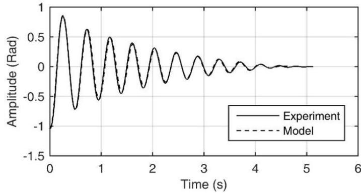
Fig. 2. Experimental results compared with numerical results based on optimization. ( $l=7.12\text{cm}$ ,  $L_{wet}=13.85\text{cm}$ ,  $h_g=1.15\text{cm}$  and  $\theta_0=1.04\text{Rad}$ )
