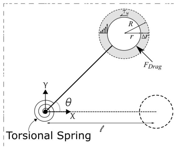
Fig. 1 Schematic diagram of the pivoted cylinder.
