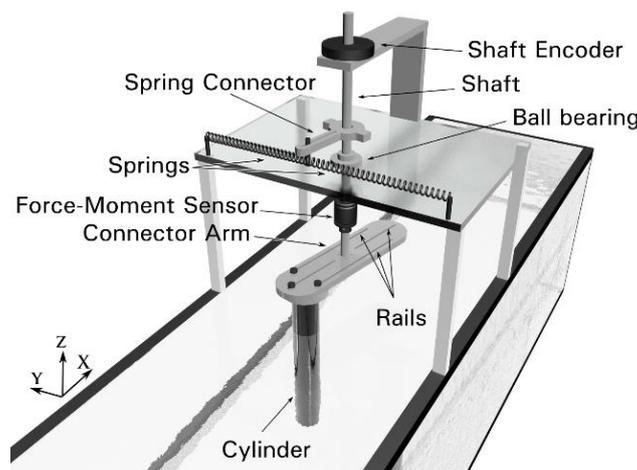
Fig. 1 3D view of experimental setup.
